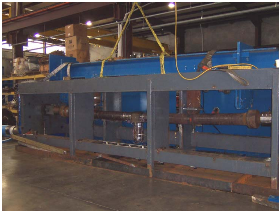
Figure 10 – Load frame used for pressure-tension-bend testing
