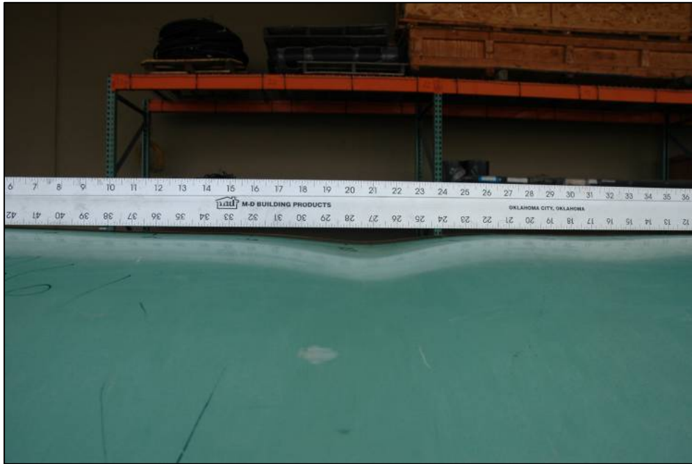
Figure 12 – Photograph of flat spot in pipe prior to cyclic pressure fatigue testing
